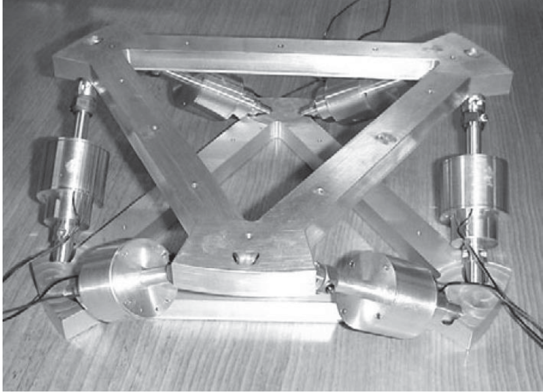
Figure 1.14: Cubic hexapod manipulator with piezoelectric actuators [36].
