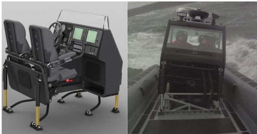
Figure 1.8: Shockwave Seat company 6-DOF isolation, marine-based occupant seating systems for rough ocean conditions.
