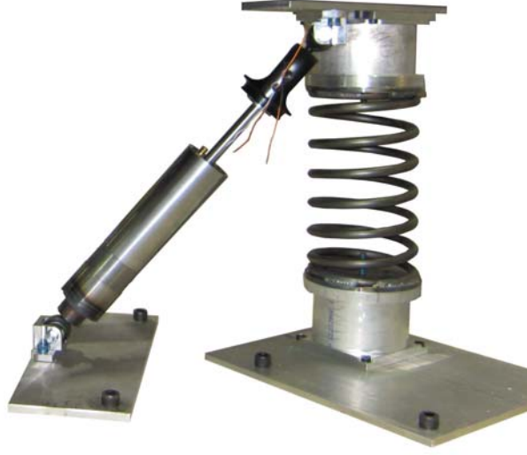
Figure 4.2: Single suspension leg.
