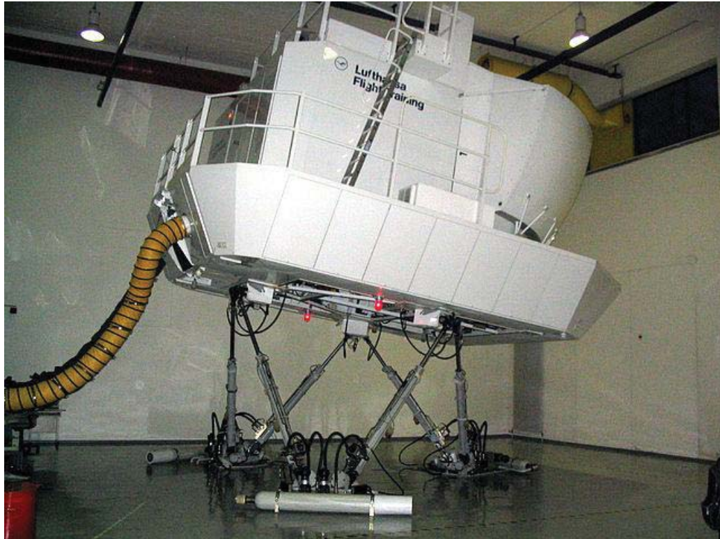
Figure 1.11: Flight simulator motion achieved with a hexapod manipulator.
